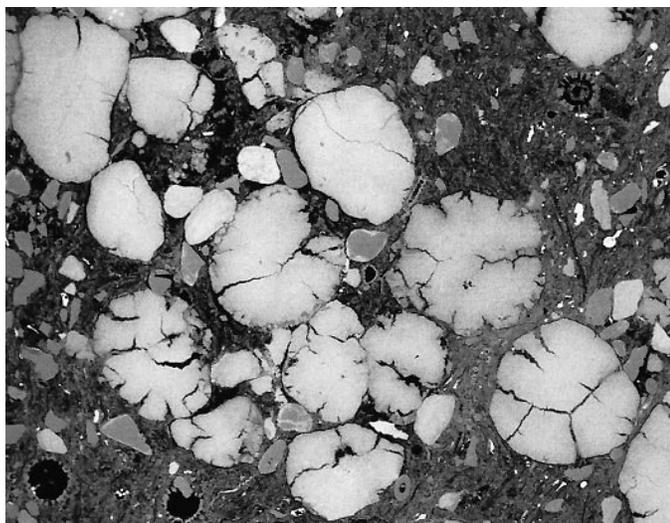
FIG. 7.—Deep-water glaucony. BSEM image of polished section at 644.88 mbsf (interval 174A-1073A-71X-1, 17–19 cm) showing high glaucony content combined with low quartz sand content. The sediment fabric is very heterogeneous with whole glaucony grains concentrated in a burrow that runs from top left to bottom right. Horizontal field of view is 1625  $\mu\text{m}$ .
