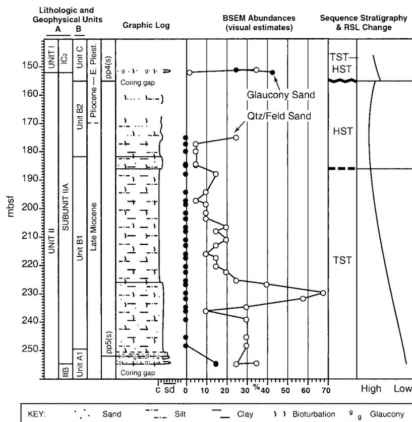
FIG. 2.—Summary of the shallow-water sedimentary succession at Site 1072 showing positions of the principal glauconitic horizons and abundances of the main sedimentary components based on visual estimate. Shipboard lithostratigraphic units (A) are from Austin et al. (1998) and lithofacies units (B) are from Metzger et al. (2000). Decreasing grain size to a maximum flooding surface at  $\sim 185$  mbsf is indicated. TST = transgressive systems tract; HST = highstand systems tract.
