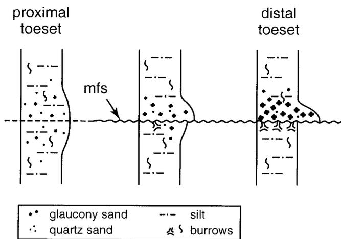
FIG. 10.—Cartoon showing hypothesized relationship between distance to clinoform front and the toset facies associated with maximum flooding surfaces (cf. Fig. 9). The proximal toset facies is characterized by small *in situ* glaucony grains mixed with common quartz sand, whereas the distal toset facies is characterized by common large *in situ* glaucony grains mixed with sparse quartz sand and is floored by a well-developed bioerosional surface. mfs = maximum flooding surface.
