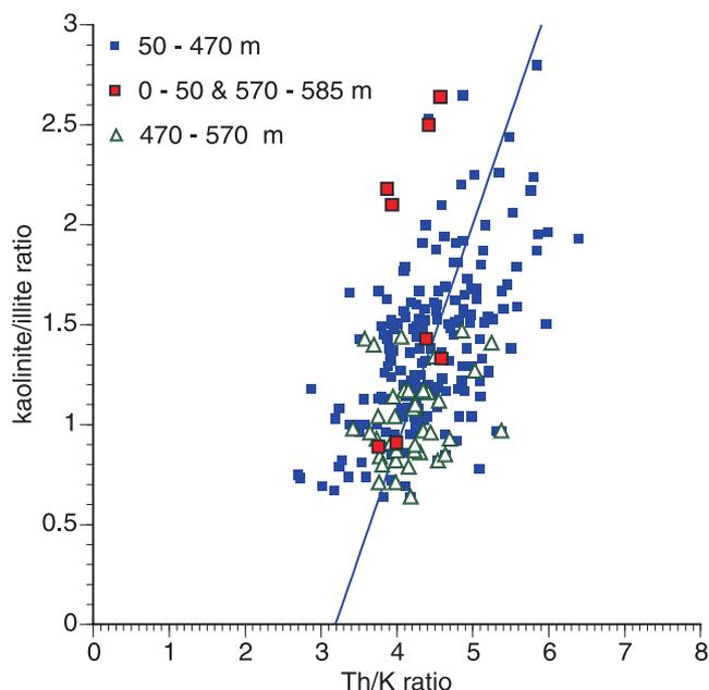
Fig. 4. Cross plot of downhole Th/K (SGR) v. kaolinite/illite (XRD) from core samples. Data points plotting well above the linear regression line ( $R^2 = 0.43$ ) are likely to contain authigenic kaolinite.
