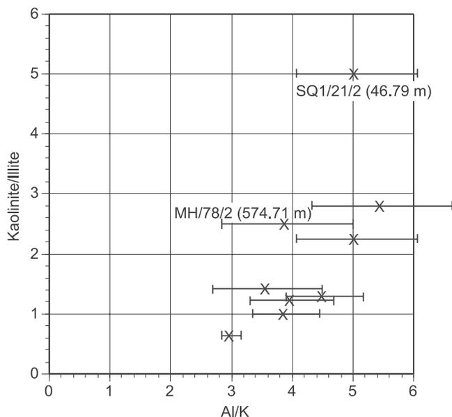
**Fig. 6.** Cross plot of Al/K (EDS) v. kaolinite/illite (XRD) for selected core samples. It should be noted that sample SQ1/21/2, 46.79 m, contains excess kaolinite over illite in comparison with Al/K values of other samples, and from BSEM images clearly contains diagenetic kaolinite (see Fig. 5a). Bars represent one standard deviation, where  $n = 5-10$ .
