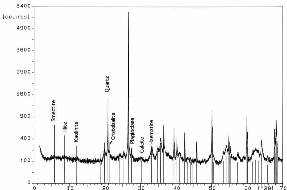
**Figure 3. X-ray diffraction trace of a clay-bearing sample of laterite from Rouge Homme, Coonawarra. The lines indicate the positions of mineral reflections and the mineral names denote the reflections used in the semi-quantitative analysis.**
