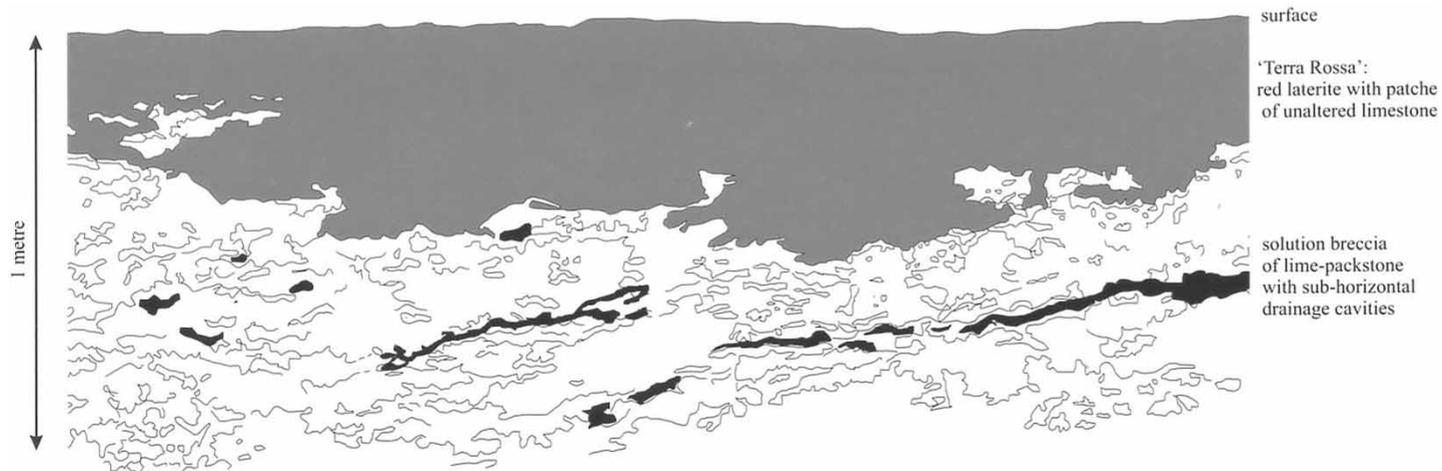
**Figure 2. Drawing of the laterite on limestone solution-breccia profile at Rouge Homme, Coonawarra; based on field sketches and photographs.**
